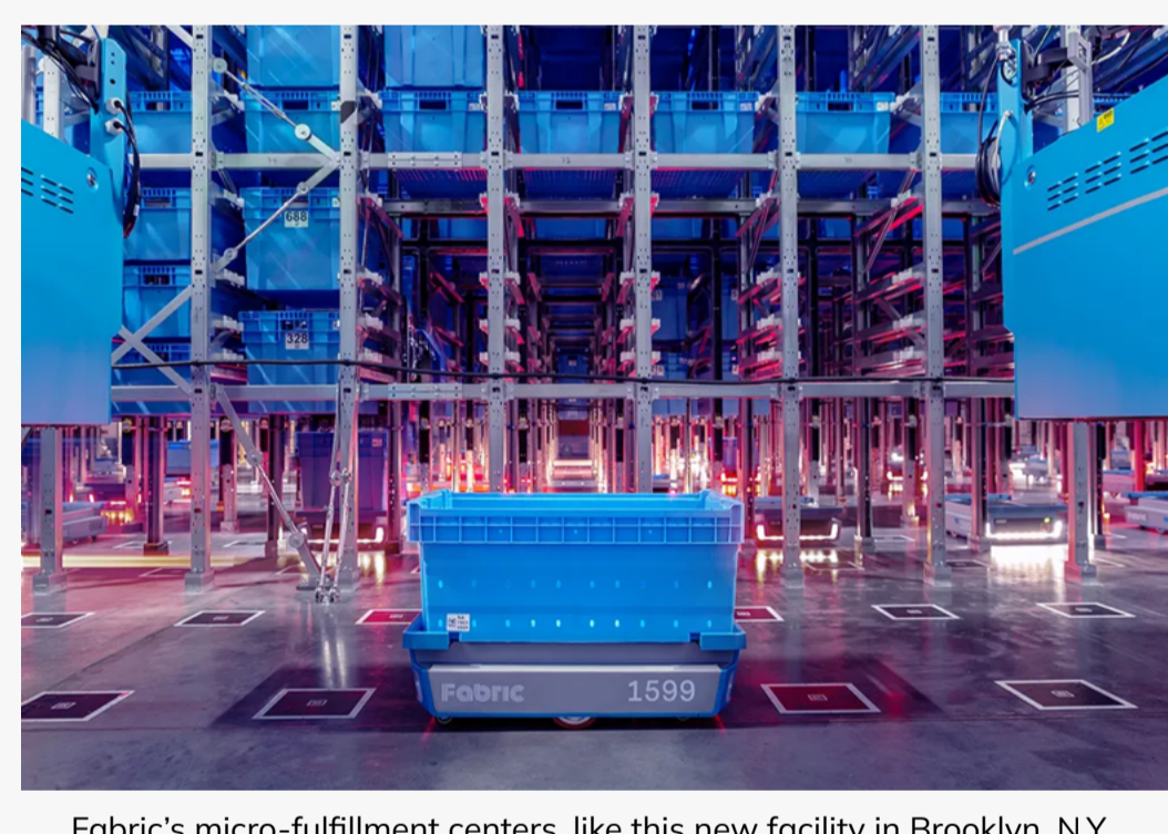
Fabric's micro-fulfillment centers, like this new facility in Brooklyn, N.Y., take up a fraction of the space of traditional automated sites, which tend to be about 10 to 20 times the size. Image courtesy of Fabric
